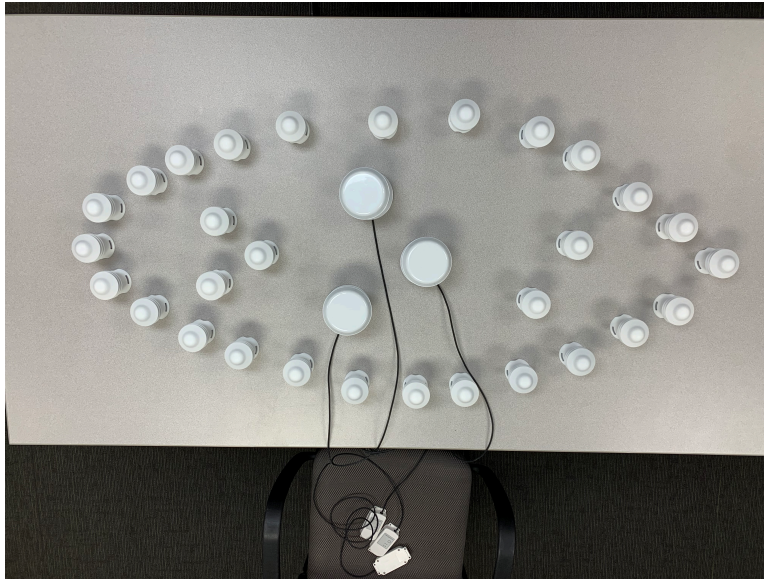
Supplementary Figure 10: Photograph of an indoor test setup for Smart-T performance evaluation. The three larger units are HOBO sensors. The other smaller units are Smart-T sensors.
